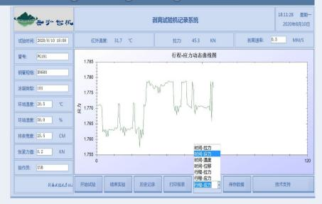
Pipeline Anticorrosive Coating Peeling Strength Tester is mainly used for testing steel pipes (3PE/PP) with external anti-corrosion treatment, and measuring the adhesion of the external anti-corrosion layer on the surface of the steel pipe, that is, the peel strength.
